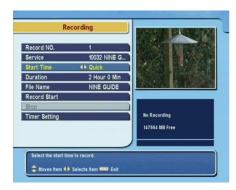
Move to Start Time and then use the left and right arrows on the remote control to change the setting to Current event. Now, move down to Record Start and press the OK key. The PVR will automatically work out how much of the programme is left to record, and set the length of the recording for you.
